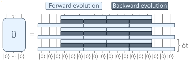
Figure B.1: The Lightcone unitary decomposition As theoretically proposed in Ref. [396], and explained in greater detail both in this appendix and in Section 10.2.4, we perform efficient Hamiltonian unitary evolution by exploiting the relatively short-ranged interaction. Specifically, we both Trotterize the unitary evolution in time, and also in space. We use a combination of forward and backwards evolution in order to keep Trotterization commutator errors to an optimal minimum.
